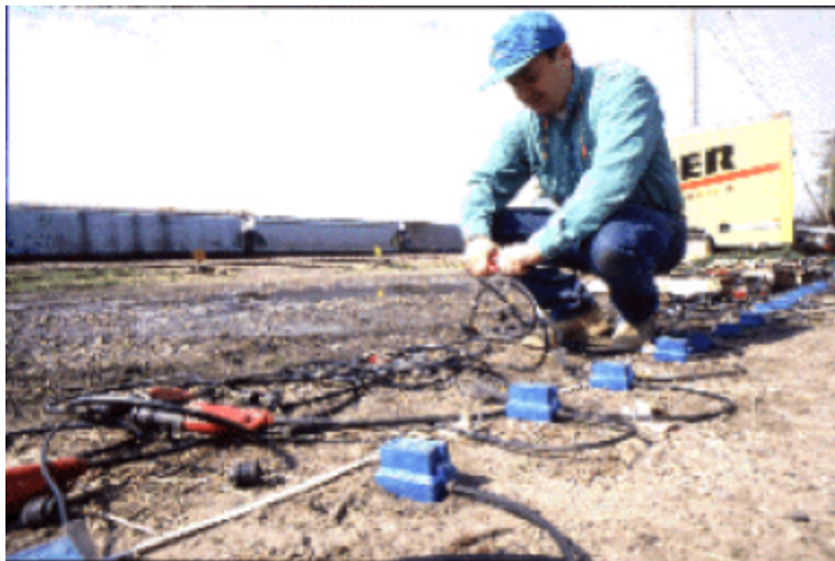
Photograph showing deployment of geophones and cable.
